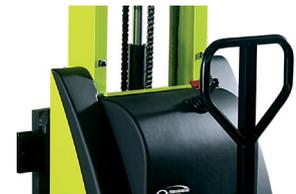
The ergonomic tiller allows excellent directionality of the machine, thanks to a steering system on both rear wheels.
