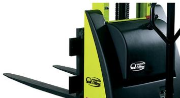
It allows an easier access to the battery housing for faster ordinary maintenance.
