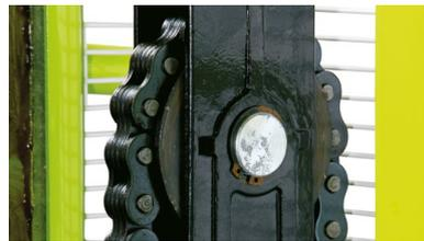
A sturdy chain and a strong steel pulley ensure great resistance and reliability even working at maximum load capacity.
