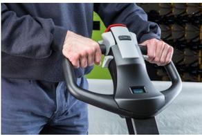
A fully integrated ergonomic tiller made of techno-polymer offers a comfortable grip. Fingertip throttle and proportional fork controls, safety push button, horn, turtle button, hour-meter, battery status indicator offered as standard equipment.
