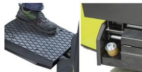
The LX stacker can be equipped with a cushioned stand-on foldable platforms and is very useful for covering medium-sized distances and for intensive application.
