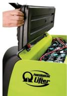
The separate battery compartment allows the installation of a high capacity battery (225Ah - 300Ah). The battery inspection is easy and comfortable via the battery cover with hinges. As an option the automatic battery refilling system can be supplied as the external high frequency battery charger that can be easily plugged trough an Anderson connector.
