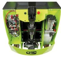
Removing the strong cover allows access to the electric and hydraulic system as well as the motorwheel and stabilizing wheels.
