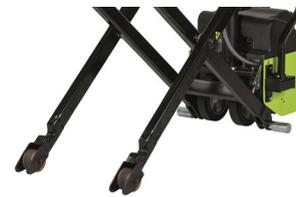
Greater machine stability achieved by using load rollers in a more advanced position and providing front and rear stabilizers as standard. The rear stabilizers, once exceeded 16" in height, make work stable and safe even in the case of heavy weights.
